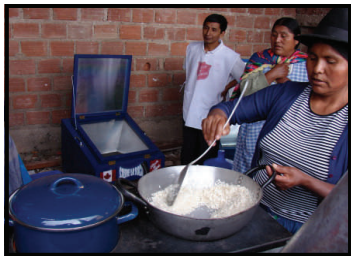
Preparing rice on a rocket stove to be cooked in a box solar cooker in retained heat mode
